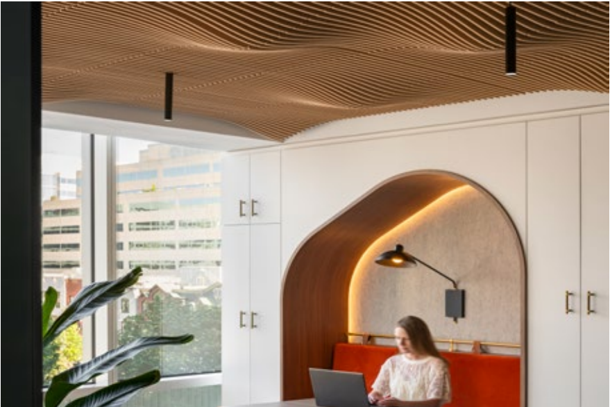
2" diameter suspended cylinder downlight with 1.5" round aperture with 0.8" light aperture regressed 0.5" from bottom of fixture.
