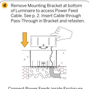
Connect Power Feeds inside Enclosure and insert Luminaire.
