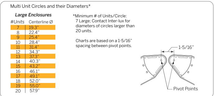
**NOTE:** Use full-size templates at end of this document to determine # of Units in circles having different unit spacings and in non-circular arcs.
