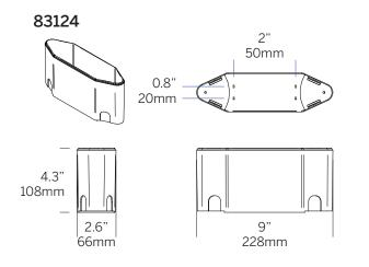
In the illustration at right, the Mounting Bracket on the back of the Luminaire is is supplied with the Rectangular Bracket attached.
