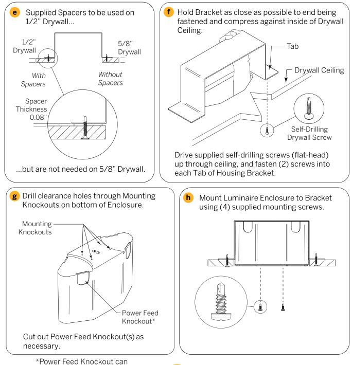
Power Feed Knockout can accept Trade Size ½ flexible conduit, having an OD of 7/8".
