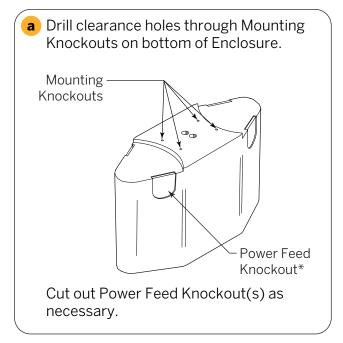
\*Power Feed Knockout can accept Trade Size ½ flexible conduit, having an OD of 7/8".
