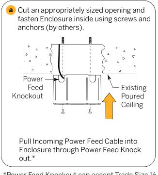
\*Power Feed Knockout can accept Trade Size ½ flexible conduit, having an OD of 7/8".
