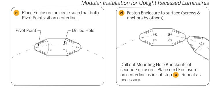
A supplied Angular Template may be used to layout multiple units in a curved run. Use supplied Pivot Hardware to maintain a uniform spacing of Enclosures.
