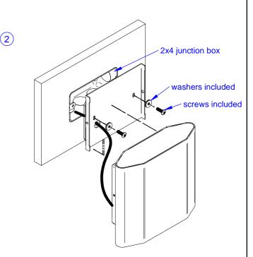
Make the wirings as shown on page 3. Install the mounting bracket on a 2x4 junction box. Connectors for splices included. Warning! Washers have a gasket on a side. The gasket should
