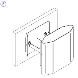
Install the fixture on the mounting bracket
