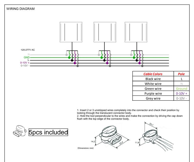
THIS PRODUCT MUST BE INSTALLED IN ACCORDANCE WITH THE APPLICABLE INSTALLATION CODE BY A PERSON FAMILIAR WITH THE CONSTRUCTION AND OPERATION OF THE PRODUCT AND THE HAZARDS INVOLVED
