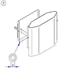
Loosen the set screw and remove the mounting bracket. Recommended tool: 2mm hex key
