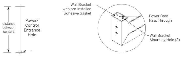
Pull Power (and Control) wires through hole.
