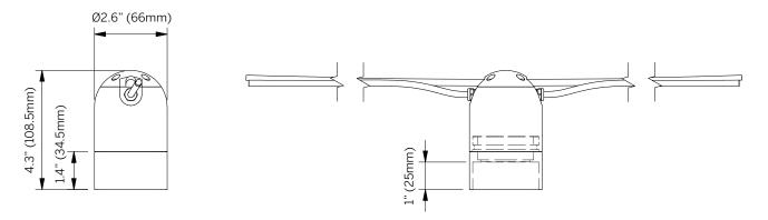
Mini G-Cat for use with a range of fixed focus optics. Fitted with low glare snoot and frosted cover glass. Provision for one external accessory.
