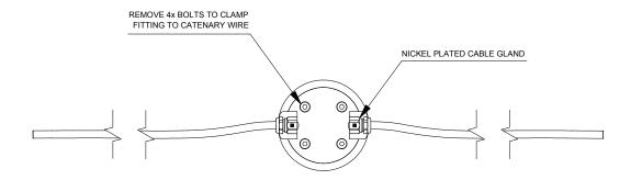
Stainless steel catenary wire removed for clarity.
