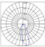
BEAM ANGLE (0-180) = 34.7° BEAM ANGLE (90-270) = 38.8°
