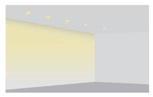
ProTools DL Wall Wash offers round and square dedicated wall wash luminaires for even illumination of a surface. They emit a wide, even beam of light which is directed towards the wall. Washlights need to be correctly positioned, both in terms of distance from the wall, and their relative distance to one another. This guide will help you get the best result.
