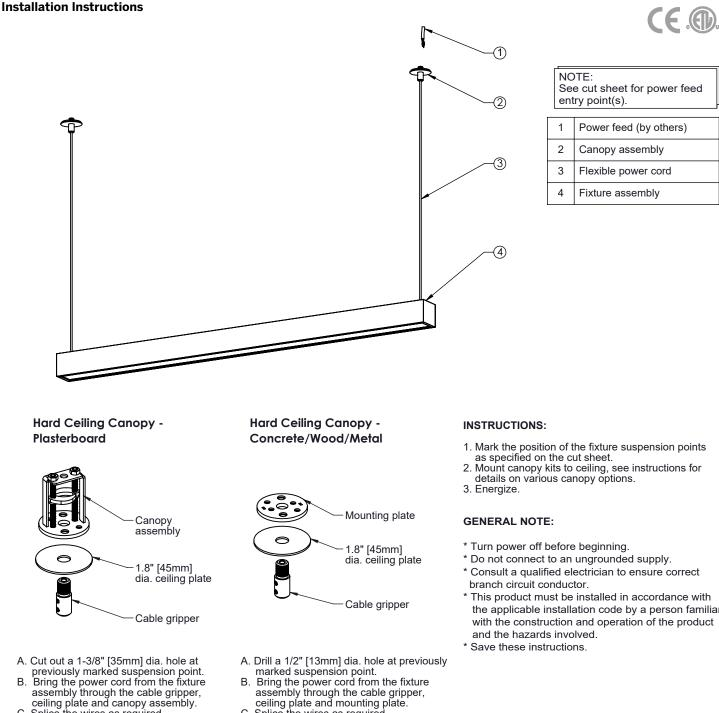
C. Splice the wires as required. Wires for connection are clearly labeled.
