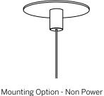
Mounting Option - Non Power Threaded Rod installed to structural ceiling (By Others)
