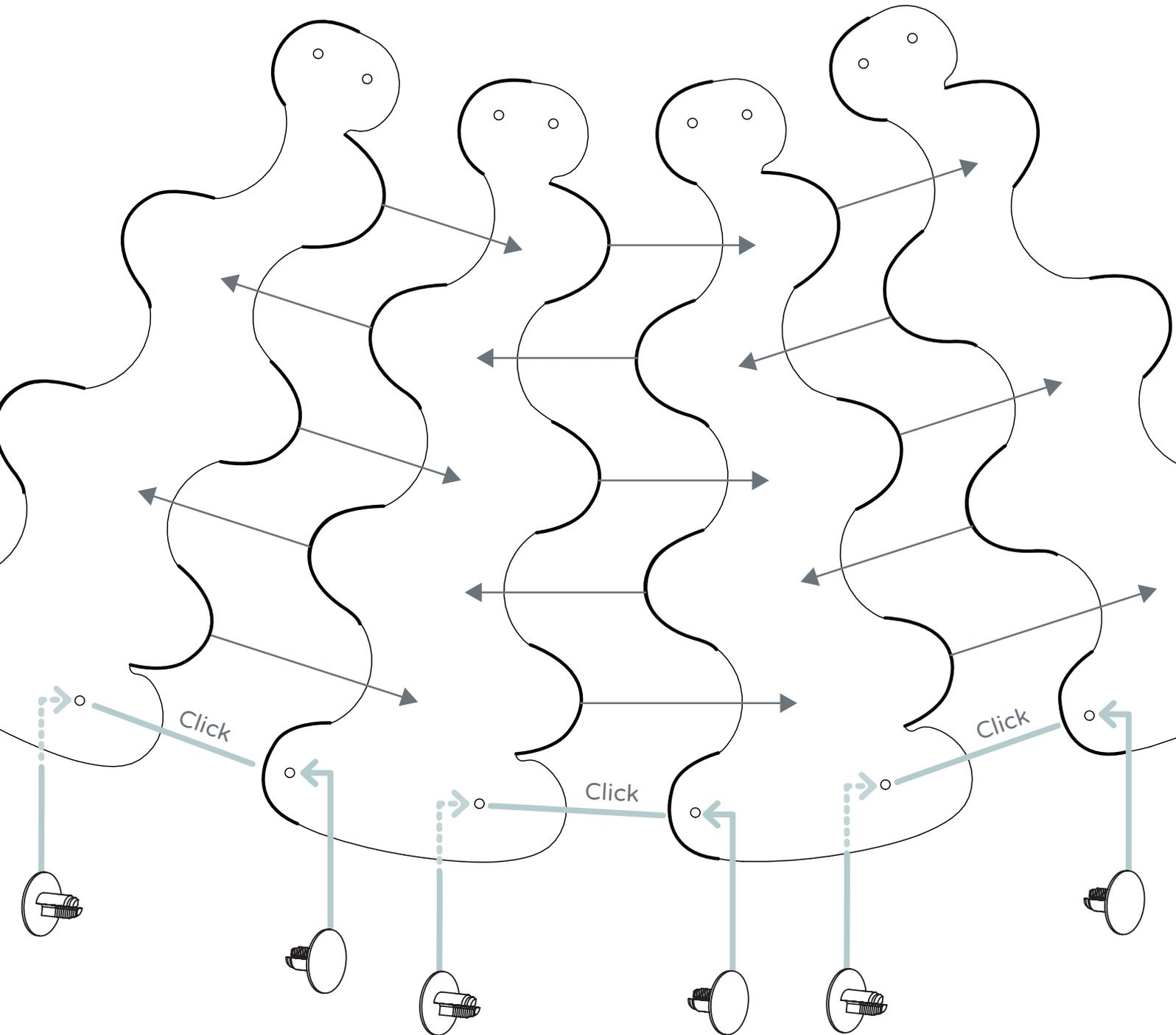
Once two panels are woven together, use two of the shorter Ratchet Rivets (13 mm) to lock them together.
