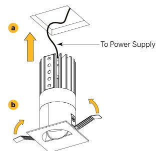
**IMPORTANT:** Add a bit of slack to power cord such that there is enough for luminaire to be fully removed without tugging on remote driver.
