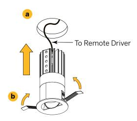
**IMPORTANT:** Add a bit of slack to power cord such that there is enough for luminaire to be fully removed without tugging on remote driver.
