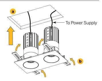
**IMPORTANT:** Add a bit of slack to power cords such that there is enough for luminaire to be fully removed without tugging on remote driver.
