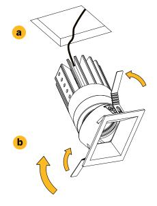
**IMPORTANT:** Add a bit of slack to power cord such that there is enough for luminaire to be fully removed without tugging on remote driver.
