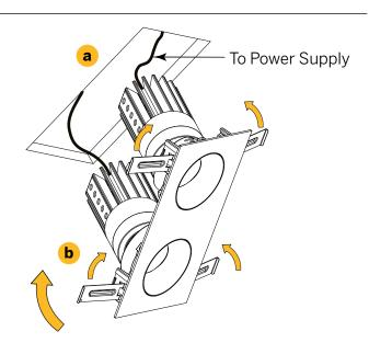
**IMPORTANT:** Add a bit of slack to power cords such that there is enough for luminaire to be fully removed without tugging on remote driver.
