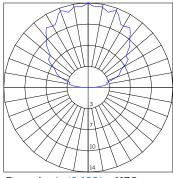
Beam Angle (0-180) = 117.8 Beam Angle (90-270) = 117.4
