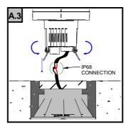
MAKE THE WIRINGS AS SHOWN IN THE WIRING DIAGRAM, OPEN THE SPRINGS AND INSERT THE FIXTURE INTO THE OUTER CASING
