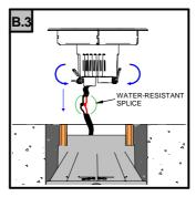
MAKE THE WIRINGS AS SHOWN IN THE WIRING DIAGRAM, OPEN THE SPRINGS AND INSERT THE FIXTURE INTO THE OUTER CASING
