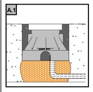
PLACE THE OUTER CASING INTO THE OPENING AND FILL THE GAP WITH CONCRETE (DARK GREY ZONE IN THE DRAWING)
