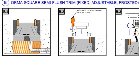
PLACE THE OUTER CASING INTO THE OPENING AND FILL THE GAP WITH CONCRETE (DARK GREY ZONE IN THE DRAWING)
