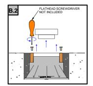
ONCE THE CONCRETE HAS SET, REMOVE THE PLASTIC SCREWS AND THE POLYSTYRENE CAP.
