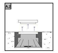
ONCE THE CONCRETE HAS SET, REMOVE THE POLYSTYRENE CAP
