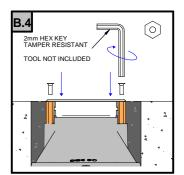
SECURE THE FLANGE WITH THE SCREWS TO COMPLETE THE INSTALLATION
