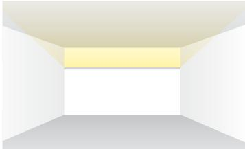
By designing a raft (ceiling cloud) in the middle of a space, the low angle light from a Whitegoods cove product can be used to illuminate the ceiling and redirect light onto adjacent vertical surfaces. A classic way to accentuate the ceiling plane can also illuminate the entire space without glare.
