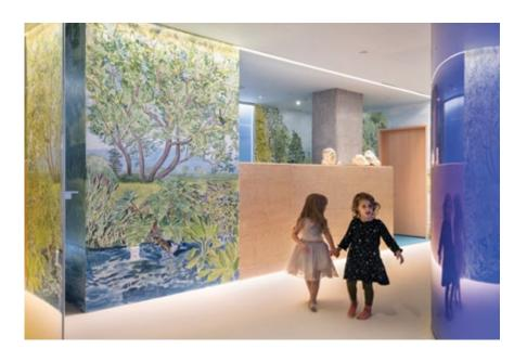
An extremely low brightness perimeter lighting system that delivers a narrow sheet of light to a feature wall from above the finished ceiling – integrated with the architecture to otherwise minimize intrusion to the space.
