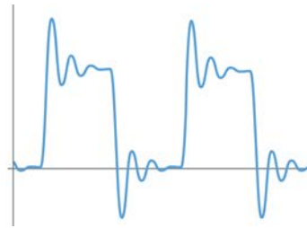
Figure 10 – Signal with reflections
