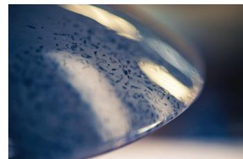
*P+AW (Powder and Acrylic Waste): 12% captured microplastic powdercoat waste, 45% granulated clear acrylic waste, 43% clear acrylic.*
