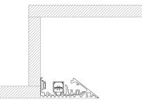
Gypsum Ceiling Mounting Options 4" minimum offset, 12" typical offset
