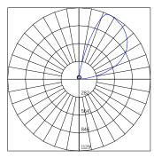
Beam Angle (0-180) = 92.7 Beam Angle (90-270) = 118.3
