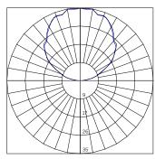
Beam Angle (0-180) = 116.5 Beam Angle (90-270) = 117.6
