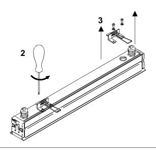
4) MOUNT THE E99818 CEILING SPRINGS KIT RESPECTING THE MEASUREMENTS BELOW. SCREWS ARE INCLUDED IN THE E99818 KIT. USE A PHILLIPS SCREWDRIVER (TOOL NOT INCLUDED) 2.95 2.95 0
