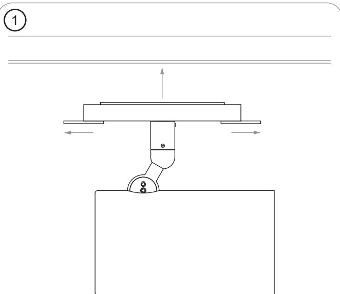
Pull out tabs to release locking grips and insert the adaptor into the track.
