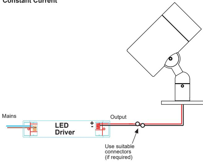
*Note that while constant current light sources can be wired in series, the number of fittings that can be wired in series is limited by the forward Voltage of the LED.*
