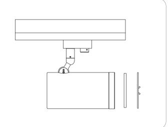
To adjust the beam angle, rotate the front section of the lamptube to the desired angle.
