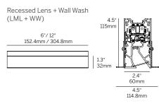
Plaster Trim Cutout Width: 3" / Length: fixture length + 1/2" Ex: 12" fixture = 12 1/2" cut out length
