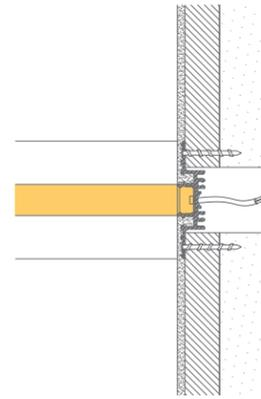
Section of Skylight Showing 20 Linear with Plaster Trim
