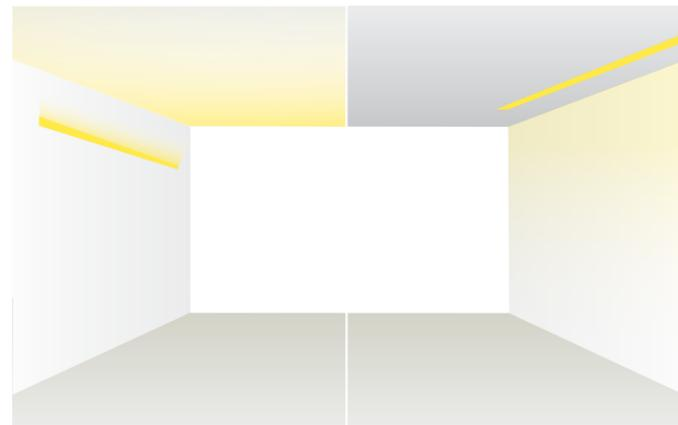
The aim of wall washing, or in fact washing any surface with light (wall, ceiling or floor), is to create an even 'wash' of light across the surface. The wall wash is a great way to introduce light into a room as the brightness of the vertical surfaces around us play a crucial role in our perception of a space. You can use linear sources which emit a wide, even beam of light directed towards the intended surface.
