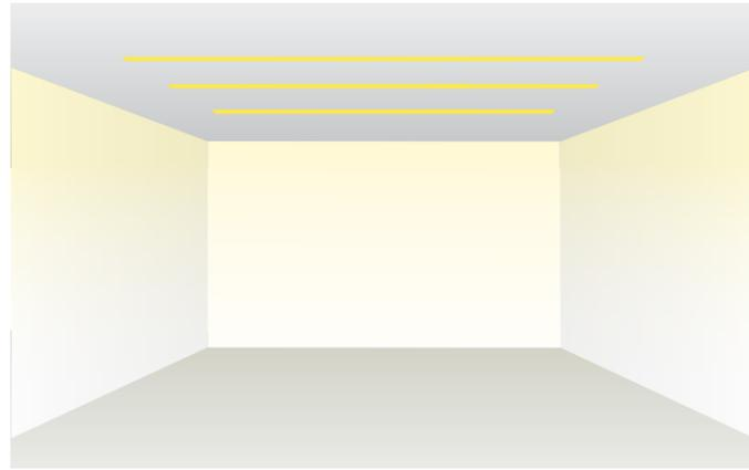
Perhaps the most common lighting solution utilized for general area lighting, arranging a group of lights in a grid to give even illumination to the surface below. Of course, the popularity of a technique is not always a sign of best practice, and in this case it typically has more to do with economy and ease of implementation.
