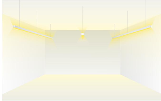
A room can be very well-lit by combining two lighting elements to achieve a perfect balance between an indirect uplight component, lifting the space and making it feel bright, and a direct component, delivering the right amount of light just where it is needed.
