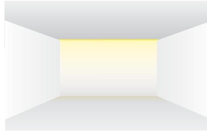
Surface Grazing is typically used to reveal and highlight textured feature surfaces such as stone, brick, wood and fabric to name a few. To achieve this, a focused narrow beam of light flows across the entire wall from top to bottom, delivering a sheet of light across the featured surface.
