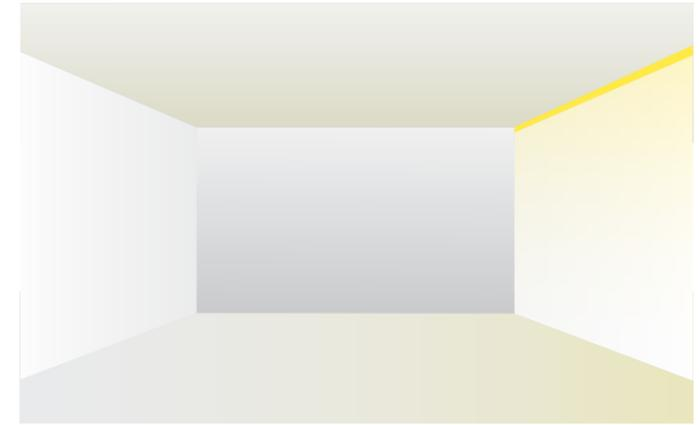
Another simple and highly effective way to add natural feeling light into a space is via a concealed linear light source detailed into the intersection of the wall and ceiling. This luminaire, typically recessed into the ceiling and providing an even illumination from a homogeneously illuminated lens, gives definition to the space, and functional light on the perimeter.
