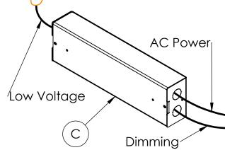
Step 3: Pull Low Voltage leads down and through wall opening. Make the connection between the Driver (C) and the AC/Dimming leads.
