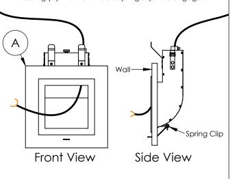
Step 5: Connect the Light Engine Insert (B) to the Low Voltage wires. Then insert Light Engine (B) into Housing (A) as shown below. Ensure that it clicks into place and that sn
