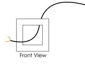
Step 4: Pull Low Voltage leads through Housing (A) and install Housing (A) into wall. Ensure spring clips are engaged.
