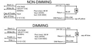
**WARNING**: if not connected to a 0-10V dimmer, driver MUST be wired as Non-dim. Not doing so can cause the driver and the fixtures to fail prematurely.
