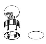
**Step 7** Push the Cover into the Insert and snap into place.
