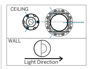
**Step 8** Push the Cover into the Insert and Snap into place observing the light orientation.
