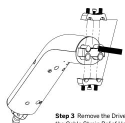
**Step 3** Remove the Driver Box cover. Loosen the Cable Strain Relief Hex Screws and Bracket. Remove the appropriate knock-outs.
