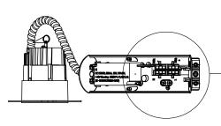
**Step 4** Connect the Feed Cable to the Black (L), White (N) and Green (Gnd) Terminals. Connect the Dimming Conductors, if applicable.
