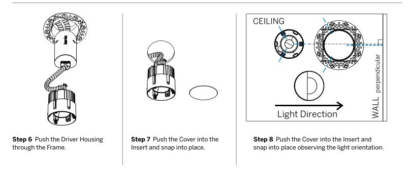
**Cover Installation** Cover should be inserted by level alignment so the (4) Touch Latches engage and hold the Cover into place. If the Cover does not engage, make sure that the Touch Latches are all OPEN (extended). When the Cover engages the Touch Latches they will be CLOSED (recessed). To remove Cover, push upward evenly and downward to release Touch Latch.
