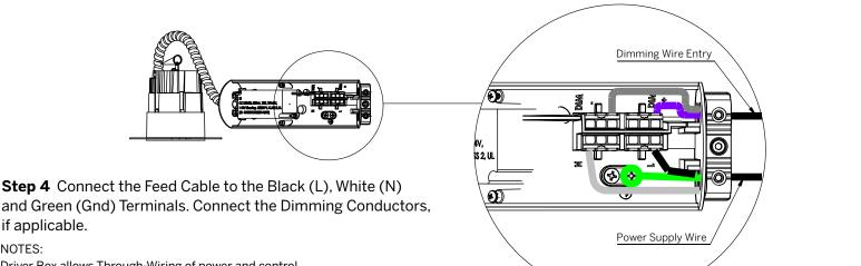
Driver Box allows Through-Wiring of power and control. Use 7/64" allen key to fix set screws. Fasten set screws provided to secure the cables as shown.
