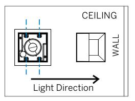
Step 9 Push the Cover into the Insert and snap into place observing the light orientation.
