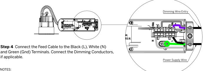
Driver Box allows Through-Wiring of power and control. Use 7/64" allen key to fix set screws. Fasten set screws provided to secure the cables as shown.
