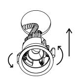
Step 7 Ensure the Wings are tight to the Housing.
