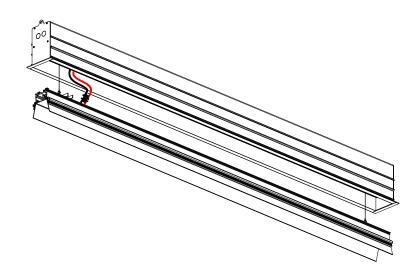
**Step 8** Connect low voltage wires from the Gear Tray to the Driver Secondary.
