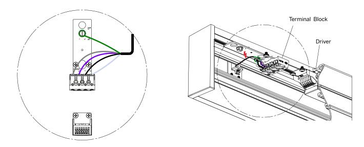
Step 7 For continuous run connect wires to Terminals as shown.
