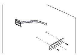
**Direct Conduit Feed** Direct 3/8" flexible conduit supply cable through Center Slot of Clips before attaching to wall.
