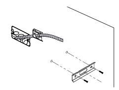
**Horizontal Switch Box Feed** Mount the Mounting Clips directly to a Single Gang j-box.
