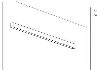
**Step 2** For continuous runs install the Joiners on to one Housing with Set Screws.
