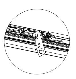
**Step 3** Pull both Tools straight down with thumbs against lens.
