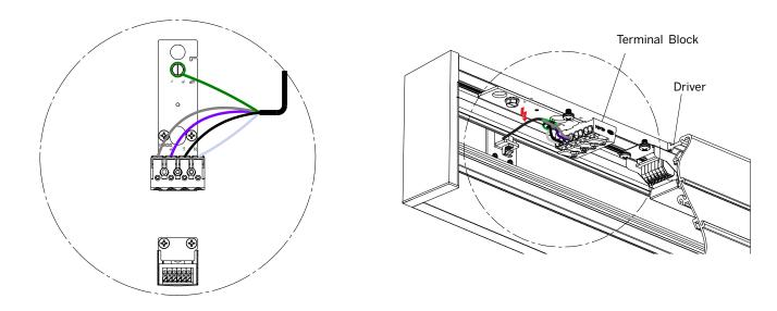
Step 9 For continuous run connect wires to Terminals as shown.
