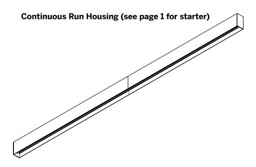
**Step 4** For continuous runs install the Joiners on to one Housing with Set Screws.
