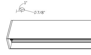
**Step 1** Cut 7/8" cable hole 1" from end of Housing.
