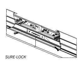
**Step 7** Attach the End Caps and tighten Set Screws ensuring there is no gap.
