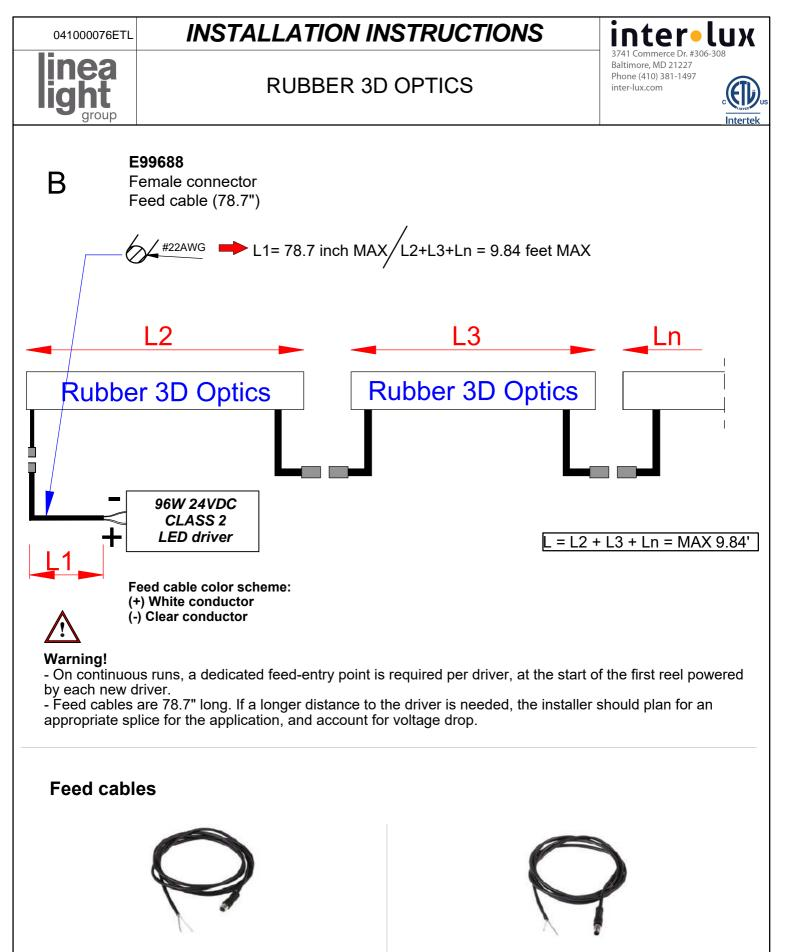
E99688 Feed Cable 78.7" 2x#22AWG
