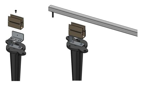
Linear profile with connector cavity Installation
