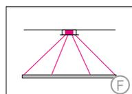
4 current-carrying steel cables. Only 1 stripe LED possible. Not in combination with RGB
