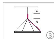
Suspension with pendant canopy and steel cables (a) 5000 mm / 196.8" + (b) 3000 mm / 118.1"
