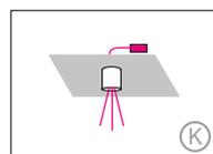
Suspension point as clamping unit with 4 current-carrying cables and remote technical unit in suspended ceiling.
