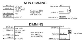
WARNING: if not connected to a 0-10V dimmer, driver MUST be wired as Non-dim. Not doing so can cause the driver and the fixtures to fail prematurely.
