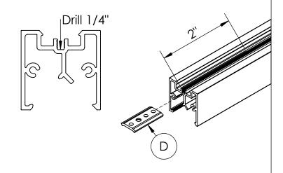
**Step 3; Install Mounting Hardware:** If installing into Tegular Ceiling tiles, assemble Tegular Extrusions (C) and Mounting Clips (F) as shown below using self tapping screws (H). Then install End Caps onto appropriate stand alone or end of run Housings (A). Finally install Snap-in Clips, and End Caps onto Luminaire (B) if required.
