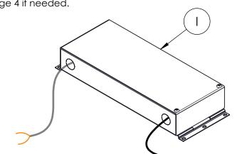
**Step 2; Prepare Housings:** Drill 1/4" diameter power feed holes in Housing(s) (A) as shown below (at least 2" from end). Then slide Joiners (D) into ends of Housing(s) (A) that will make up the joints of a continuous run (*See Step 3*).
