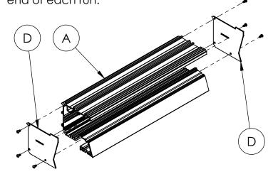
**Step 4; Installation of Joiners:** If your order consists of stand alone fixtures, skip this step. If not, connect Housings (A) to each other using supplied Joiner Kits (C). Slide pins into square holes and push Housings (A) together, then center Joiner on the joint and drive screws in Joiner as shown below.
