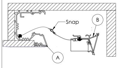
Step 11; Wiring Installation: Pull AC wires through holes on false ceiling and Housing (A). Connect the AC wires to wires of Driver located on Gear Tray (B).
