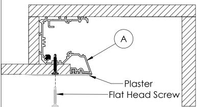
Step 7; Installation of Housing for open ceiling version: In case of open ceiling version, align and insert the Housing (A) into ceiling as shown below.
