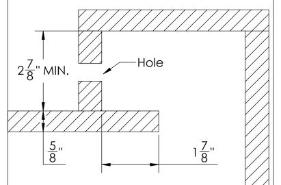
Step 2; Prepare the Housing for Installation:  $A\frac{7}{8}$
