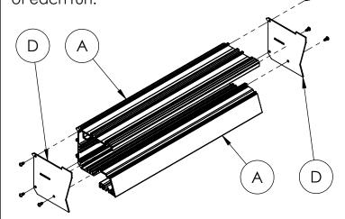
**Step 4**; **Installation of Joiners**: If your order consists of stand alone fixtures, skip this step. If not, connect Housings (A) to each other using supplied Joiner Kits (C). Slide Joiner (C) into square holes and push Housings (A) together, then center Joiner on the joint and drive screws in Joiner as shown below.
