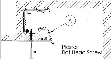
Step 7; Installation of Housing for open ceiling version: In case of open ceiling version, align and insert the Housing (A) into ceiling as shown below. Then, secure Housing (A) flange to false ceiling by using Flat Head screws for every 16" of housing as shown below. Apply plaster over the bottom side of Housing (A) and exposed screw head.
