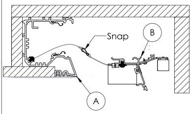
Step 11; Wiring Installation: Pull AC wires through holes on false ceiling and Housing (A). Connect the AC wires to wires of Driver located on Gear Tray (B).
