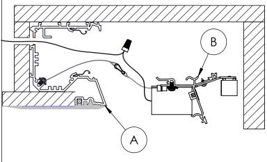
Step 12; Installation of Gear Tray and testing. Gently insert the Gear Tray (B) into Housing (A)
