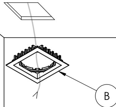
**Step 3; Installation of Housing** Push Housing (B) up into ceiling hole. Then, push Mounting Clips (C) down into slots of Housing (B) as shown below. Make sure that all three clips are pushed down until the housing is secured in the ceiling.
