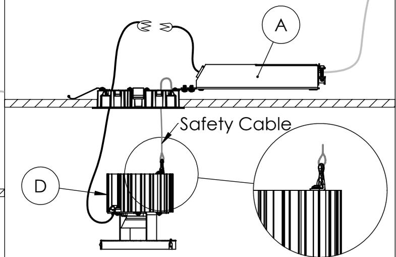
**Step 7; Installation of Light Engine:** Push the Light Engine (D) up into opening of the Housing (B) until it locks into place. Make sure pin of Housing (B) enters between fins of Light Engine (D).
