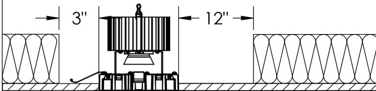
**Step 2; Wiring:** Pull AC Power, and dimming leads if required, through ceiling hole and Housing (B)
