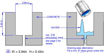
Draining pipe alternative: Fill a min. 6" deep grove under the casing with 3/4" gravel
