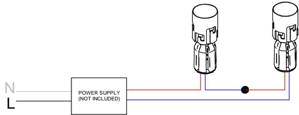
The number of fixtures on a single output will vary depending on the specific LED driver. Refer to the specific wiring diagram on <https://www.inter-lux.com/wiring-diagrams/> and the Constant Current Fixtures per driver table
