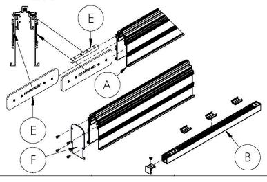
Step 4; Prepare Housings: Determine which end Luminaires (B) will be located at in Housings (A). Then drill 1/4" feed holes through Housings (A) as shown below which will line up with Low voltage cables. Next attach Hanger Brackets (D) to Housing (A) using supplied screws.
