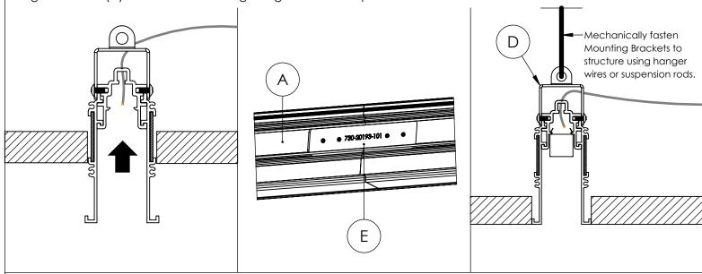
**Step 6; Install Luminaires:** Connect Luminaires (B) to Low Voltage Cables. Then install Luminaires (B) by pushing them up until they snap into Housings (A). If possible, arrange Luminaire (B) lenses so that they overlap fixture joints. Finally, power Luminaires (B) to double check electrical connections.
