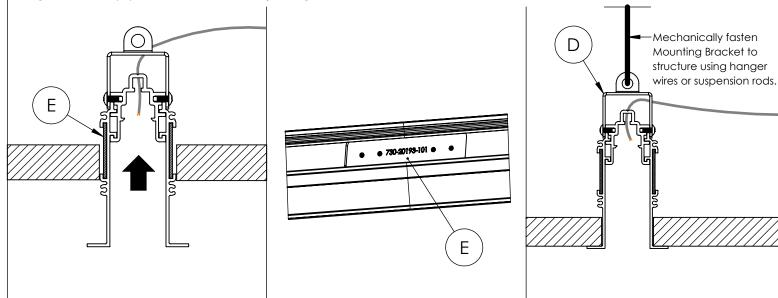
**Step 6; Install Luminaires:** Connect Luminaires (B) to Low Voltage Cables. Then install Luminaires (B) by pushing them up until they snap into Housings (A). If possible, arrange Luminaire (B) lenses so that they overlap fixture joints. Finally, power the Luminaires (B) to double check electrical connections.
