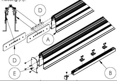
**Step 4; Prepare Housings:** Determine which end the Luminaire (B) will be located at in the Housing (A). Then drill 1/4" feed holes through Housings (A) as shown below which will line up with Low voltage cables. Next attach Hanger Brackets (D) to Housing (A) using supplied screws. Then pull Low Voltage wires through feed holes.
