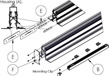
**Step 4; Prepare Housings:** Determine which end the Luminaire (B) cables will be located at in the Housing (A). Then drill 1/4" feed holes through Housings (A) as shown below, which will line up with Low voltage cables. Next attach Hanger Brackets (C) to Housings (A) using supplied M4 screws (D).
