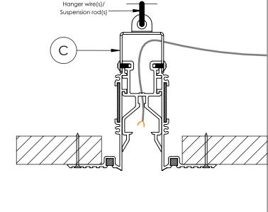
**Step 6; Install Luminaires:** Connect Luminaires (B) to Low Voltage Cables. Then install Luminaires (B) by pushing them up until they snap into Housings (A). If possible, arrange Luminaire (B) lenses so that they overlap fixture joints. Then plaster over flanges as shown below. Finally, power the Luminaires (B) to double check electrical connections.
